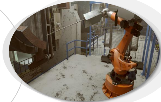
New robotic product for ladle make up area
